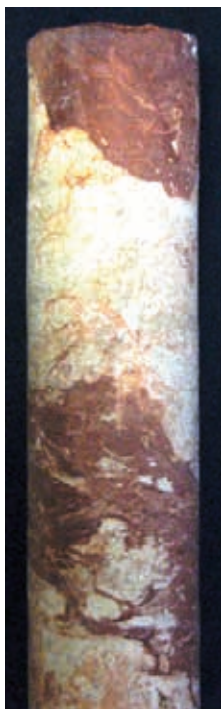
Fig. 4 app. 2 - Detail of a coring in the Triassic limestones of Halimba (Hungary): infiltration of bauxites resediment in freatic zone. From Minszenty et al., 2000. Authorized reproduction.
